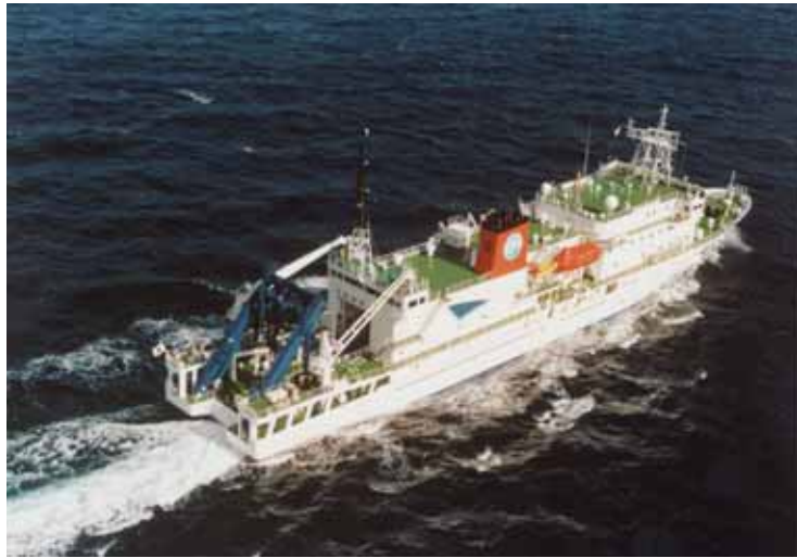
R.V Kairei 4628 tons Streamer Cable 156ch, 5000m Airgun 200 liter
