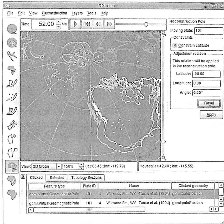
Figure 7.5. Modifying a plate reconstruction in GPlates using the interactive Modify Reconstruction Pole tool. Paleomagnetic data are being used to align the plates, so it is helpful to constrain the latitude of the plate; only the longitude of the plate will change. See color plates section.
