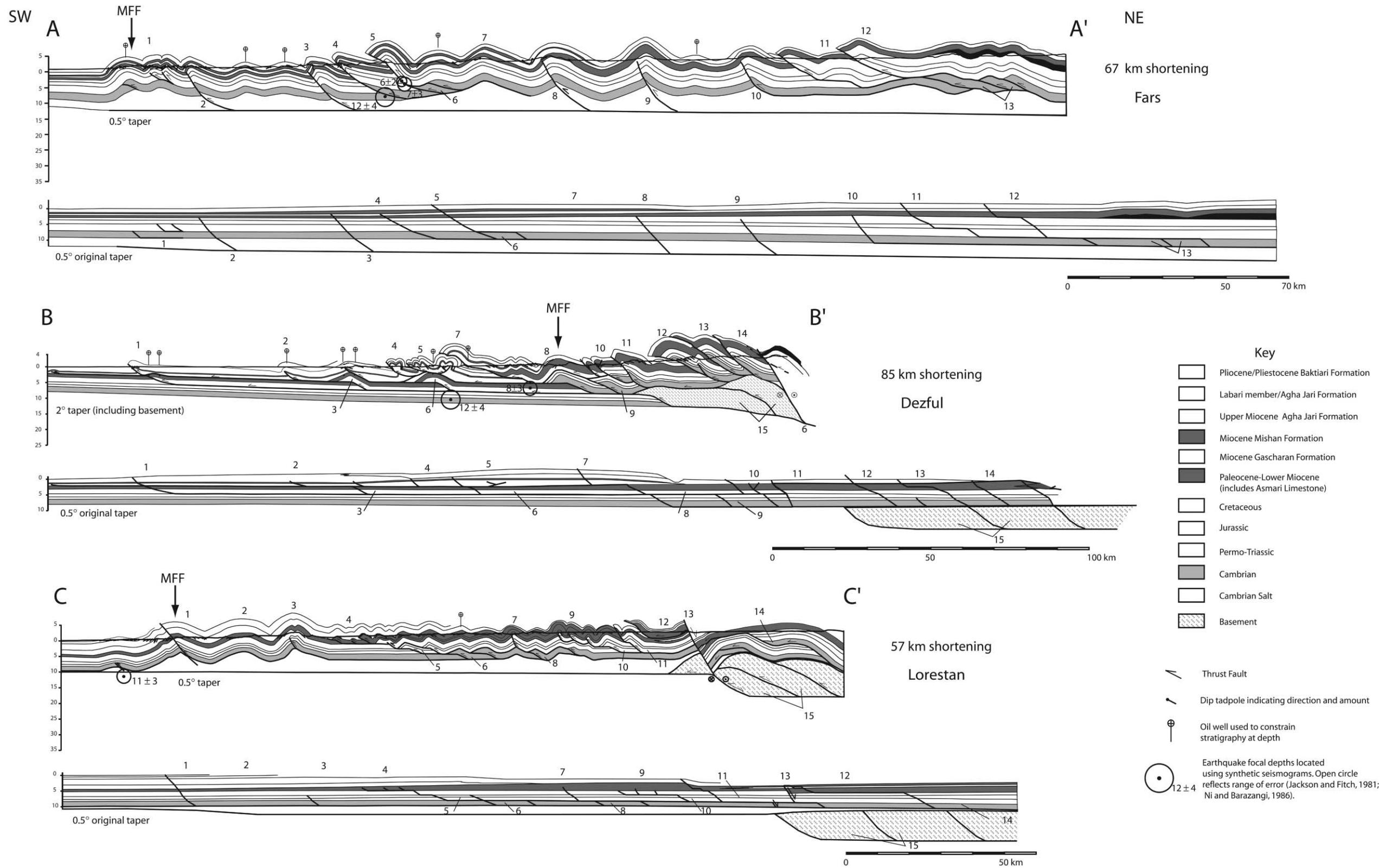
Fig. 3. Cross-sections through the Zagros fold-thrust belt. Numbers in cross-sections match numbers on restored sections and represent structures referred to in the text. See Fig. 1 for locations.
