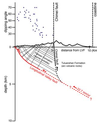
Figure B4. Reconstruction of the subsurface geometry of the Longitudinal Valley fault near Hsiukulan canyon, from bedrock dip angles. The azimuth of the section is approximately N80W. This model indicates that the dip-slip rate along the fault is about 22.7 mm/yr and that all of the deformation is accommodated by the slip along the fault plane, with no internal deformation of the beds.
