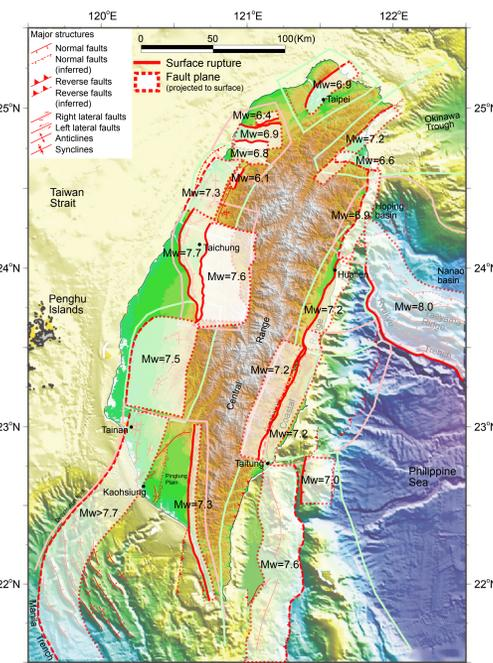
Figure A2. Proposed major sources for future large earthquakes in and around Taiwan. Bold red lines are proposed future ruptures, and the white patches are rupture planes projected to the surface. Here we have selected only a few representative scenarios to show in this figure. Earthquake magnitude of each scenario is predicted value from our calculation.
