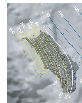
The uplift pattern in 2005 broadly mimics the shape and location of Nias island: the welt of maximum uplift is along the west coast and the line of zero uplift approximately follows the east coast. Will some increment of 2005 uplift be preserved as permanent deformation? With the support of the Tectonics Observatory and NSF, we are currently studying uplifted fossil coral reefs around the margin of Nias to address this question.
