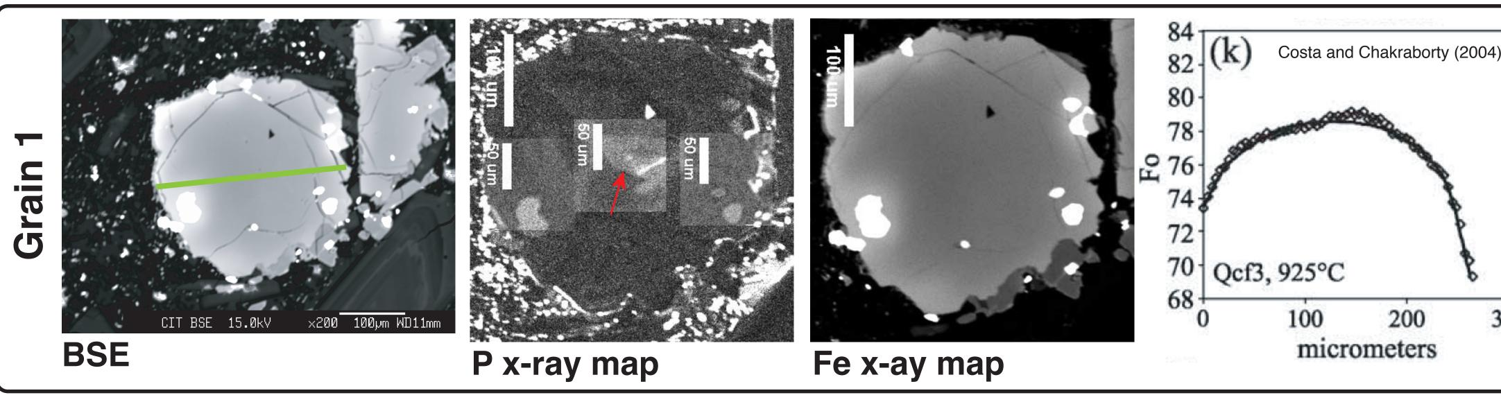
These grains do not have good crystal faces. The red arrows on the P x-ray map point to features in the P<sub>2</sub>O<sub>5</sub> zoning region. The  $P_2O_5$  zoning is patchy in the interior of the grain (Grains 1 and 2); grain 2 also has a suggestion of  $P_2O_5$  banding near the edge of the crystal. The green lines on the BSE images correspond to the Fo profiles.
